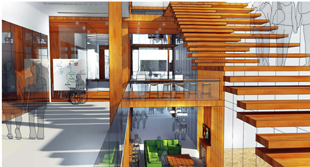
An early design concept for Western Oregon University's College of Education building calls for the use of cross-laminated timber in stair treads. (Mahlum Architects)
