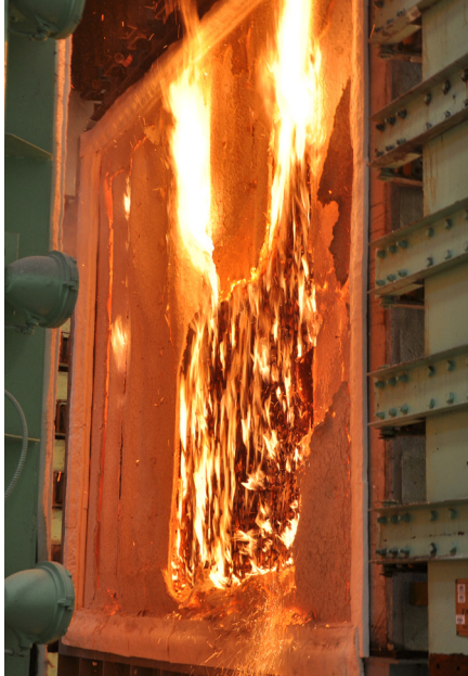
Fire testing CLT wall assembly. Image: FPIInnovations
