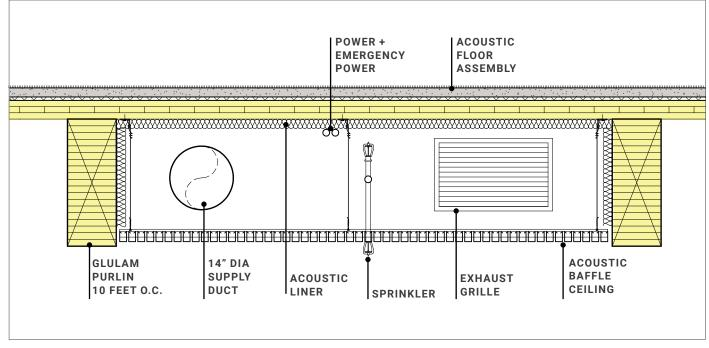
ABOVE: Section through acoustical suspended ceiling assembly
