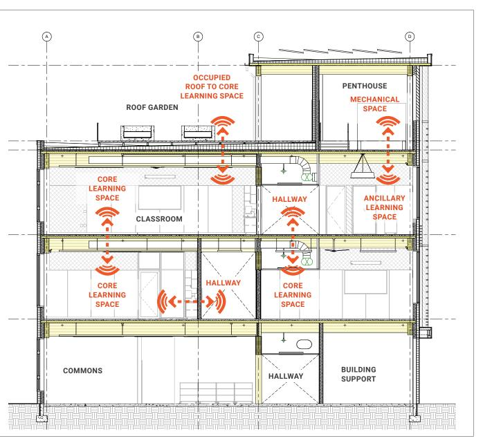
ABOVE: Building section showing key acoustic partition types
