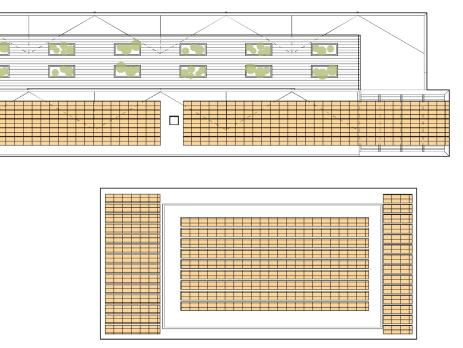
ABOVE: Roof plan showing extent of roof-top PVs on classroom building (top) and pavilion (bottom)
