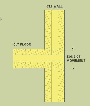
perpendicular to growth rings, creates intermediate dimensional change. The smallest amount of dimensional change is that which occurs along the axis of the tree, parallel to its grain. Mass timber elements that utilize adhesive bonds between laminations, like CLT and GLT, generally have good dimensional stability.
