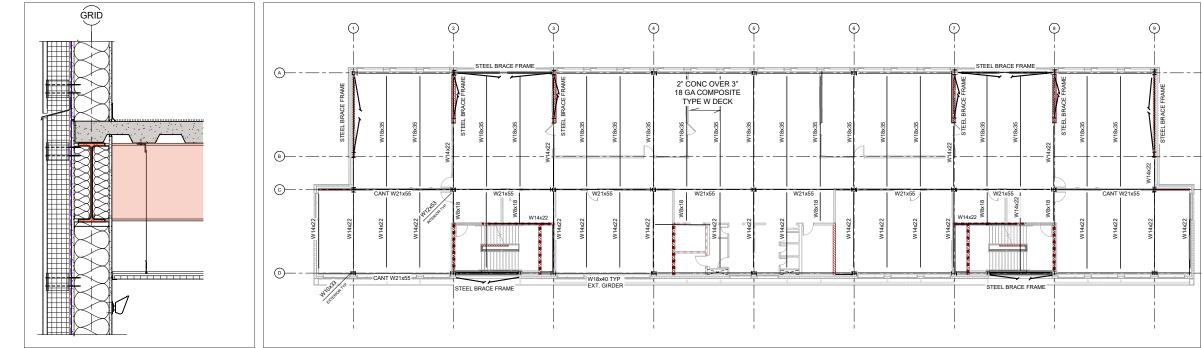
ABOVE: Exterior wall, steel construction detail. ABOVE: Steel framing plan for typical upper floor.
