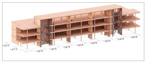
ABOVE: Vertical, horizontal, bracing, and CLT structure
