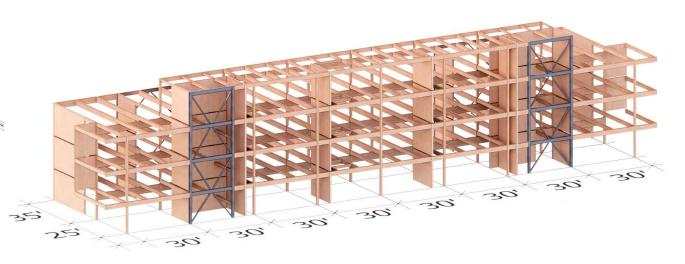
ABOVE: Mass timber structural framework with steel brace frames and CLT shear walls designed for flexibility. (CLT floor and roof deck not shown for clarity.)
