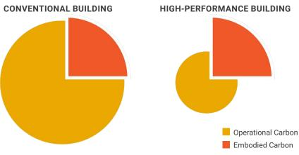
ABOVE: As buildings become more energy efficient, embodied carbon represents a larger share of the overall climate impacts over a building's life due to GHG emissions related to construction and construction materials
