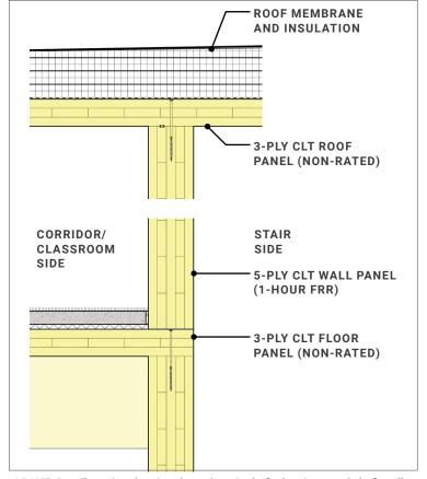
ABOVE: Detail section drawing through stair shaft showing rated shaft wall and intersection of non-rated floor and non-rated roof (While this detail meets continuity requirements of building code, its acceptance should be confirmed by the Authority Having Jurisdiction)
