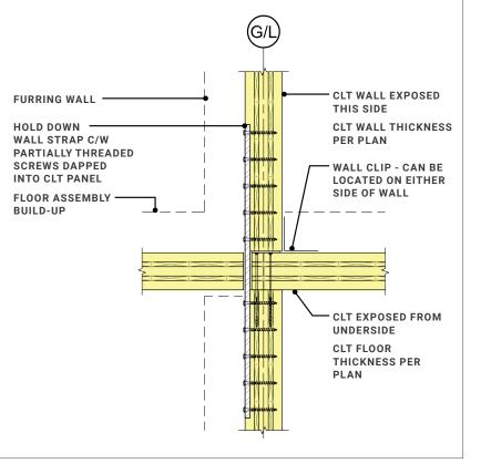
ABOVE: Typical Floor-to-Floor Hold Down Splice Section Detail
