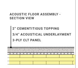
In this project, the gypsum-based topping layers noted above may alternatively consist of concrete of the same thickness. Regardless of whether gypsum-based topping or concrete topping is used, the buildups will still require an acoustical underlayment of the same thickness noted previously. Email correspondence with the USG Corp. indicated that use of gypsumbased topping in lieu concrete could reduce embodied carbon emissions for identical thickness.7
