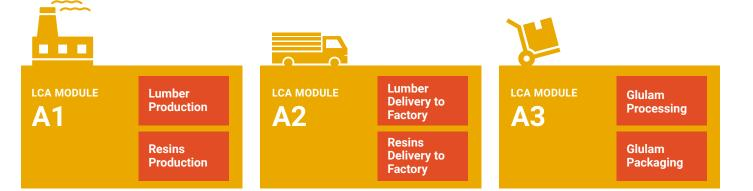
ABOVE: Cradle-to-gate LCA modules for glulam production.
