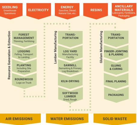
ABOVE: Cradle-to-gate inputs and outputs from glued laminated timber production.
