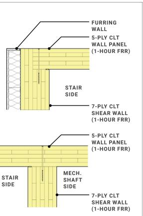
Plan details showing CLT intersections at stair shaft (FRR = Fire-Resistance Rated)
