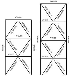
ABOVE: Brace frame elevations for building's north side (left) and south side (right)
