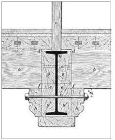
ABOVE: Wood insulates a steel beam in traditional heavy timber floor construction to protect it in the event of a fire. (See the **Building Code** section for more information on fire resistance and contemporary practices.)
